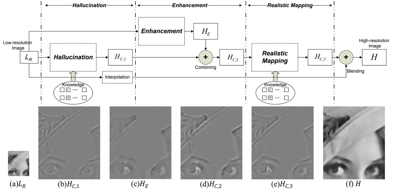
Figure 3: Our image hallucination framework: (a) the input low-resolution image  $L_R$ ; (b) high-frequency component  $H_{C,1}$  hallucinated by [3]; (c) high-frequency component  $H_E$  generated in Enhancement tier; (d) enhanced high-frequency component  $H_{C,2}$ ; (e) target high-resolution component  $H_{C,3}$  with our model.
